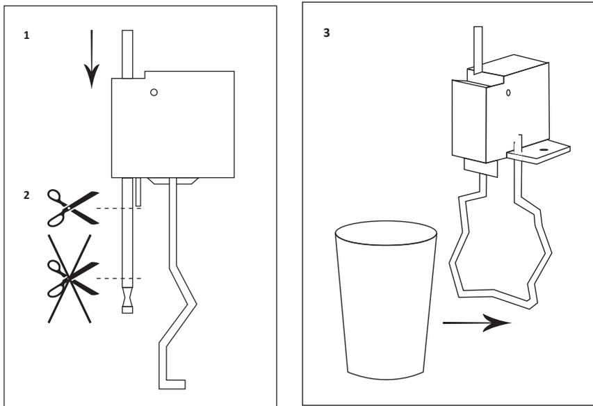
Open the doors of the device and place the bag into the device with the hose pointing downwards and to the front, so that the bag is centred over one of the two or three taps.
